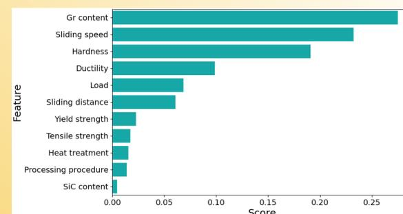
Fig.5. Feature importance in wear rate prediction
