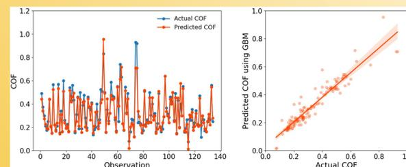
Fig.2. Predicted COF using GBM vs actual COF
