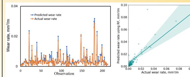
Fig.3. Predicted wear rate using RF vs actual wear rate
