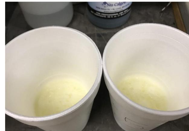
Figure 6: Polyurethane foam with collapse < 15mm
