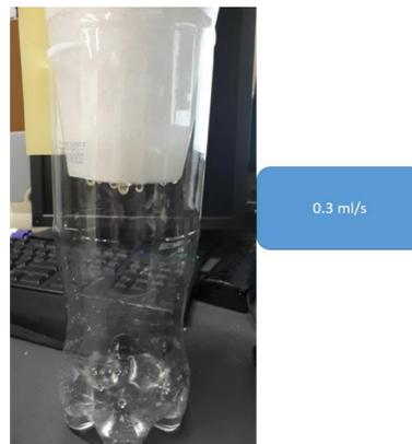
Figure 5: Permeability testing
