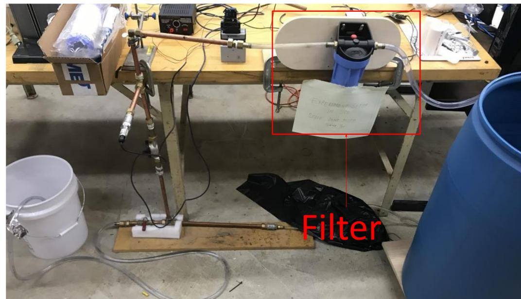
Figure 7: Arsenic removal set up
