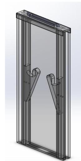
Figure 3 – Submergent Nozzle Design
