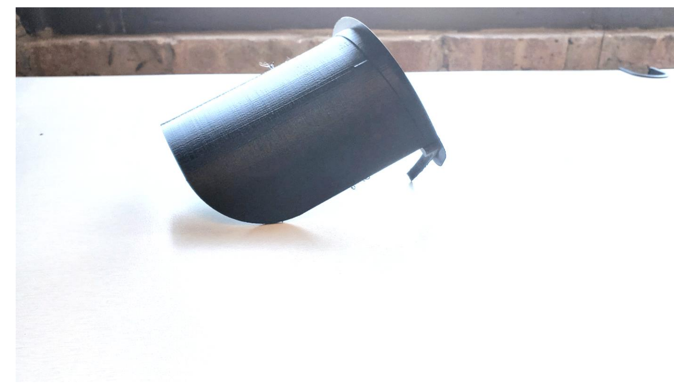
Figure 3: Prototype of 3D printed face shield in the lab. Transparent material for face portion should be used for practical use
