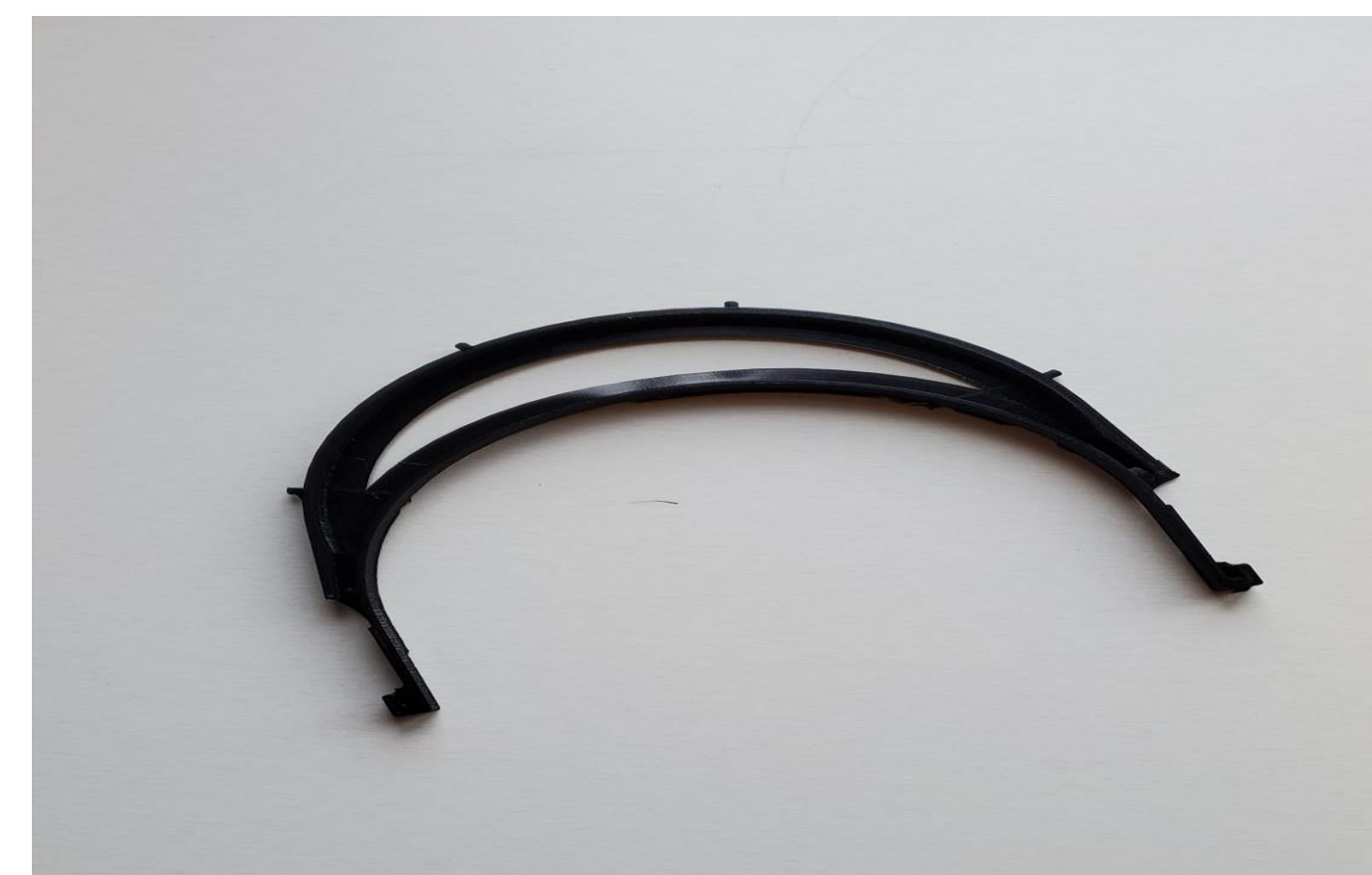
Figure 4: Prototype of 3D printed face shield band. A plastic cover can be attached with it for the extended portion
