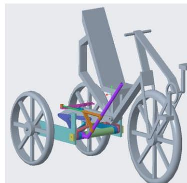
Full Assembly Model of Cruzbike Q45 with Tilting Trike Bracket and Tilt Control User Interface
