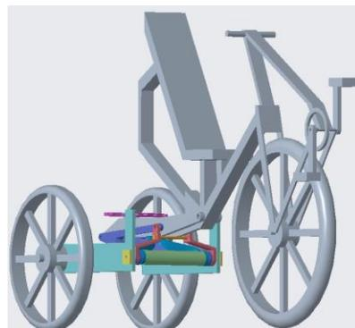
Full Assembly Model of Cruzbike Q45 with Tilting Trike Bracket
