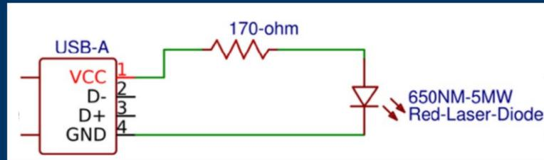
Fig.3 Custom-made circuit used to power the laser for DIHM
