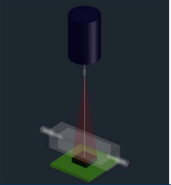
Fig.2 Laser (top), cuvette, and CMOS (bottom) work together
