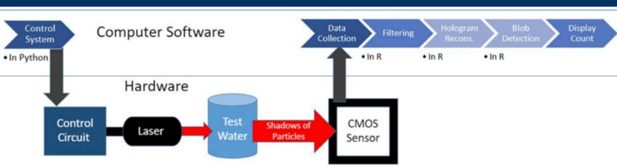
Fig.1 Particle sensor design
