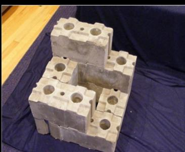
Image of AIMU blocks made of CLC and stacked to show interlocking capabilities for zero lateral movement.
