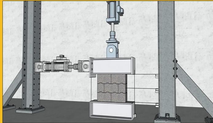
Figure 1: Test of dry-stackable AIMU blocks for local crushing properties using two flat top and bottom blocks, with two regular blocks in the center.
