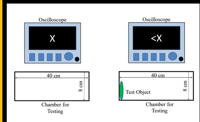
Figure 3 | Schematic of the testing environment – a visual representation of how the data is interpreted.
