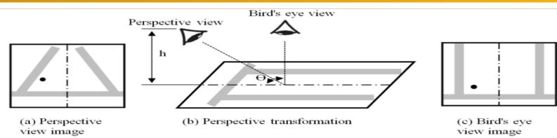
Figure 2. A perspective image transformation to a bird's eye image
