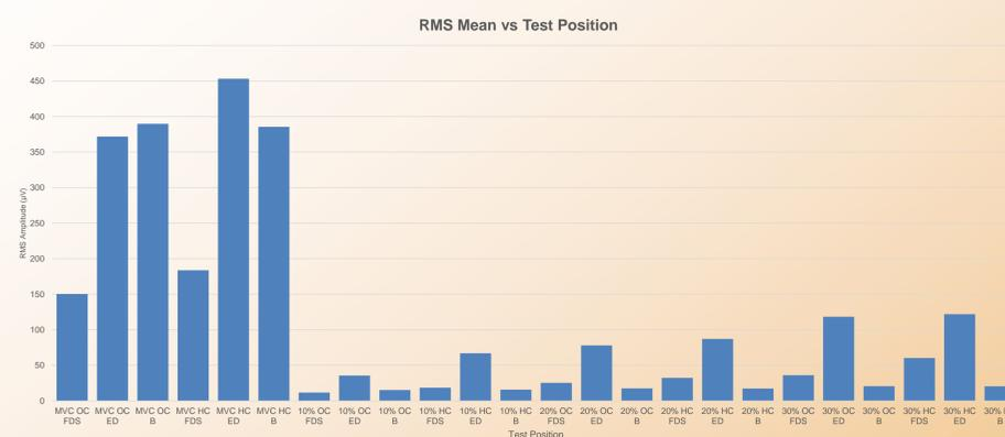
Figure 5: Bar Graph of the Mean RMS amplitude collected from the EMG sensors attached to the subject in each of the tests
