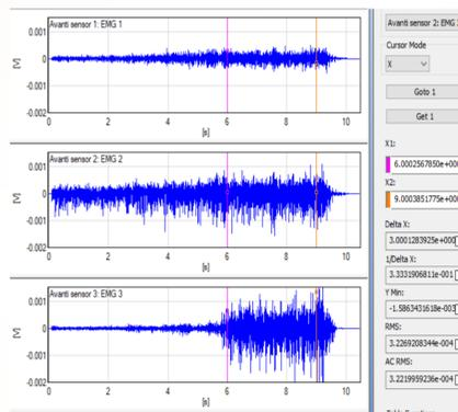
Figure 3: Example of EMG signals obtained from the subject. Cursors indicate the interval over which data was collected
