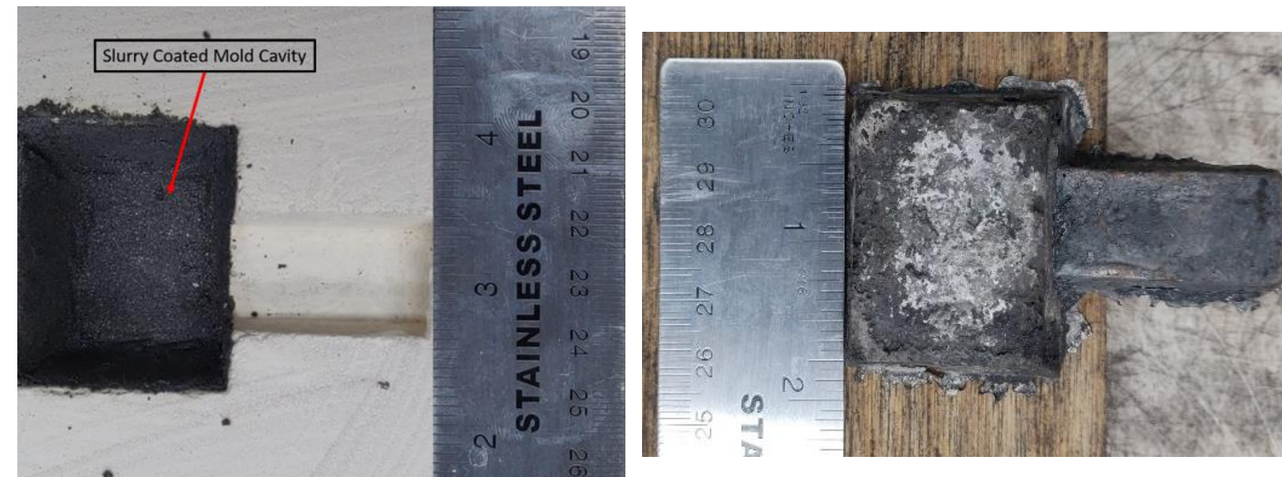
Fig 1. Mold cavity coated with slurry of alloying powder and binder
