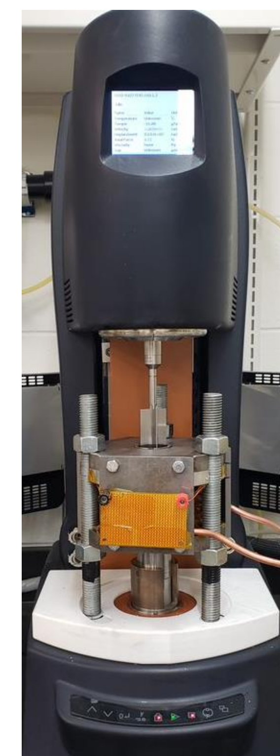
Fig. 2. Magnetorheological setup using an electromagnet
