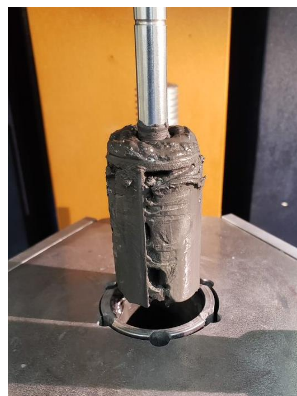
Fig. 3. Stiffening of mortar from a previously fluid mixture after MF exposure
