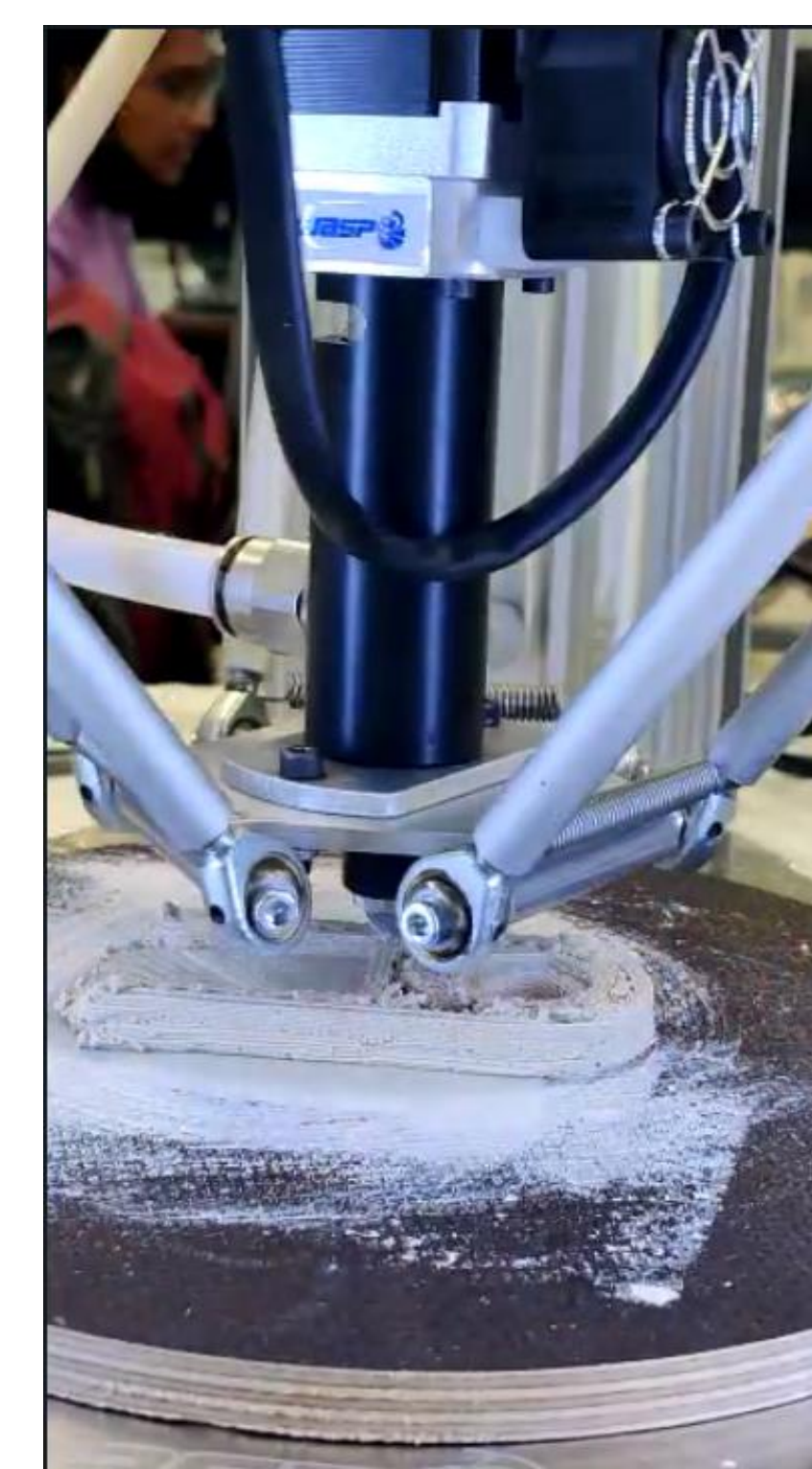
Fig. 4. Preliminary test print using a clay 3D printer
