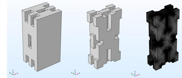
Figure5. Unit-cell and fluid domain geometries and refined generated mesh
