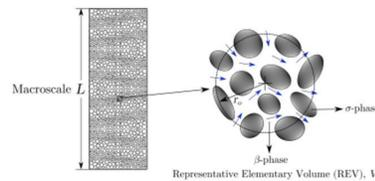
Figure3. Sketch of a macroscopic region of length L and a spherical Representative Elementary Volume (REV) of volume V with radius  $r_0$ . The REV is composed of solid ( $\sigma$ ) and fluid ( $\beta$ ) phases.
