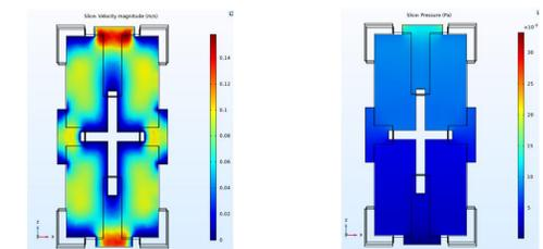
Figure7. Velocity and Pressure contours in the mid plane of the unit-cell
