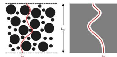
Figure4. Flow path within a porous medium
